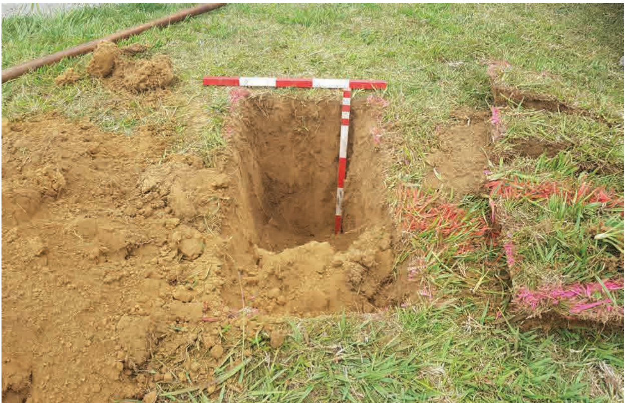
Figure 5. Pothole on top of S15/235 showing thin topsoil onto loam. Photo scales = 0.5 m.
